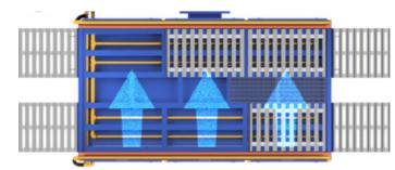
**SELF CLEANING** Isolated pipe flushes heavy particles from the base unit
